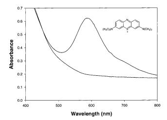
**Figure 3.** Absorption spectra in the region of 400 to 800 nm for (A) TEA $-MnO_x$  film and (B) MB $-MnO_x$  film.
