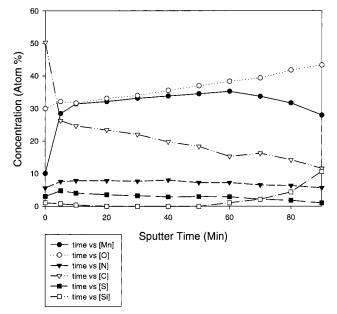
**Figure 1.** XPS depth profile of  $Cd-MnO_x$  film.
