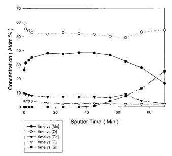
**Figure 2.** XPS depth profile of  $MB-MnO_x$  film.
